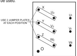
Figure 26. Voltage Change-Over Board 480V Configuration
